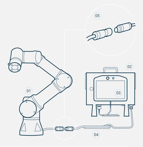
Every e-Series purchase includes a 6 m standard cable and a base flange connector that enables through-side and through-hole mounting for your robot.
